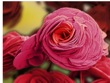
SEM image of a catalyst for the production of maleic anhydride (magnification 9000x)- Nano Imaging Lab, SNI, University of Basel
