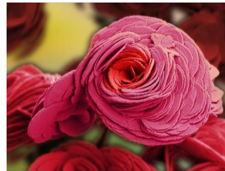
SEM image of a catalyst for the production of maleic anhydride (magnification 9000x)- Nano Imaging Lab, SNI, University of Basel
